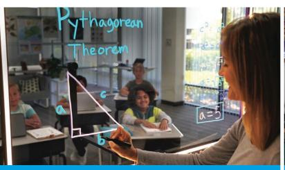
The built-in camera captures your face and writing in the same frame, and flips the image so text reads correctly.
